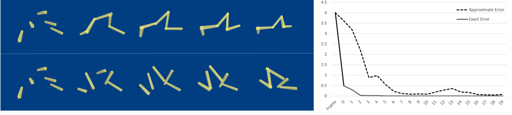
Fig. 2. Convergence of a system of bodies and joints comparing the difference between using a linear approximation of the constraint error in the Gauss-Seidel update vs. using an exact update in a non-linear version of a Gauss-Seidel update, as discussed in section 4.1. The initial configuration presents a challenge to the solver, as it requires large rotations of the bodies in order to fix all of the constraints. Note: in these tests the solver is using 10 iterations in both cases, and the error in the exact case can be reduced further by increasing the number of iterations, unlike with the linear approximation, where the solver can diverge if there are large errors.
