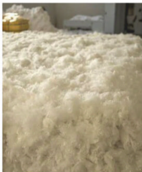
Fibre blending at the Pure Waste factory. The opened, blended fibres (below) are then spun (below-centre)
