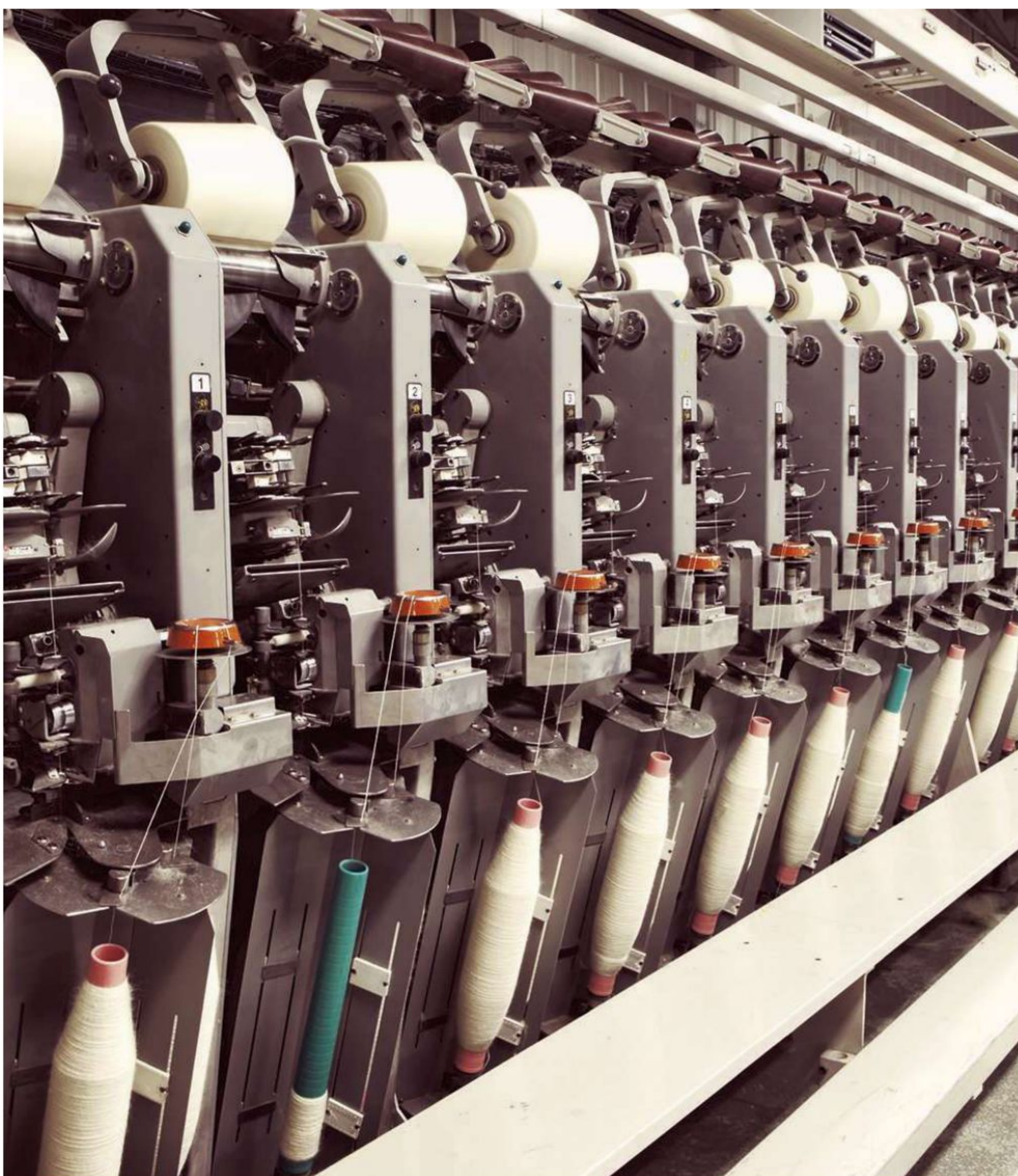
Opposite: Scrummy Signature 4ply yarn by West Yorkshire Spinners in the Spice Rack colour palette. This page, clockwise from left: The Muratec Murata machine cleverly maintains an even diameter of yarn; bundles of wool tops waiting to be processed; the natural, undyed range of 100% Bluefaced Leicester wool.
