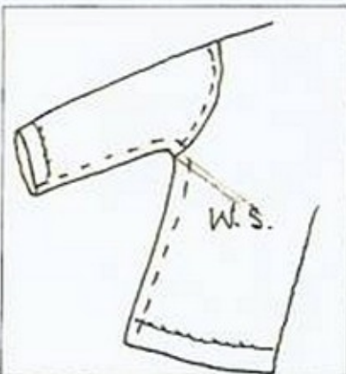
11 Sew the side seams. Hem the sleeves and jacket.
