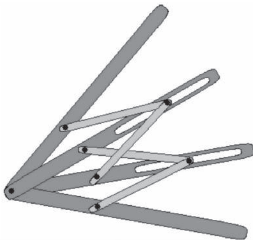
A linkage for trisecting angles.
