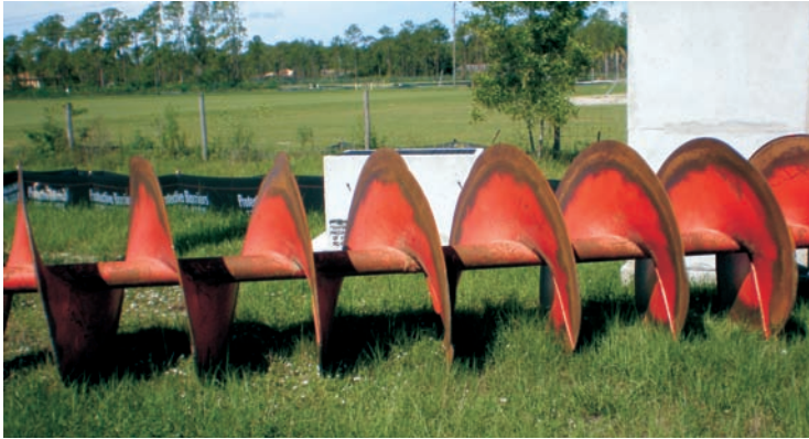
Contemporary auger at a construction site that is the same Archimedean screw still used after more than 2000 years.
