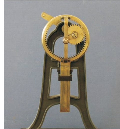
Planetary gear or Tusi couple mechanism, Kinematic Model Collection, Cornell University (photo by Prof. Francis Moon).
